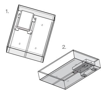
**Shelf Mounting:** The EL-SC-150 has rubber feet to protect finished surfaces. Set the controller in a location that will allow you to properly manage connected wiring so that there is no tension on the connections.
