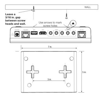
NOTE: Mounting height < 2 meters. Weight < 1 kg.
