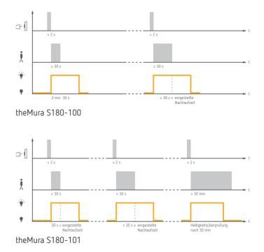
When the button is pressed briefly, the light switches on for a certain time (depending on the duration of motion and the set time delay).
