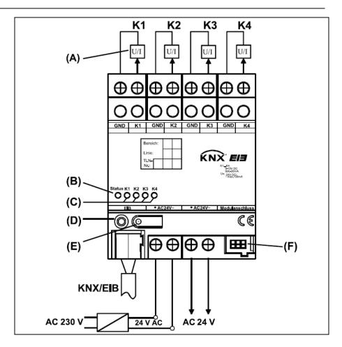
GND: reference potential for outputs K1 ... K4
