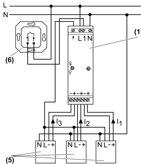
picture 2: Connection diagram, single-phase
