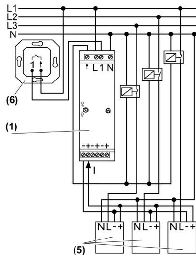
picture 3: Connection diagram, three-phase
